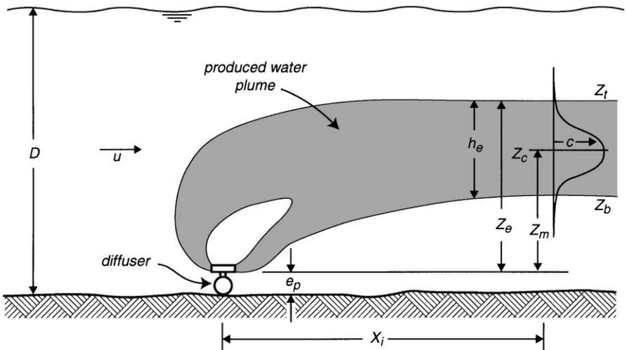
Fig. 2. Diagram of a buoyant produced water plume released from a multi-port diffuser on the seafloor (adapted from Baumgartner et al., 1994). Produce water is discharged through tee-ports on diffuser and spreads as a buoyant plume. See text for explanation of symbols.
