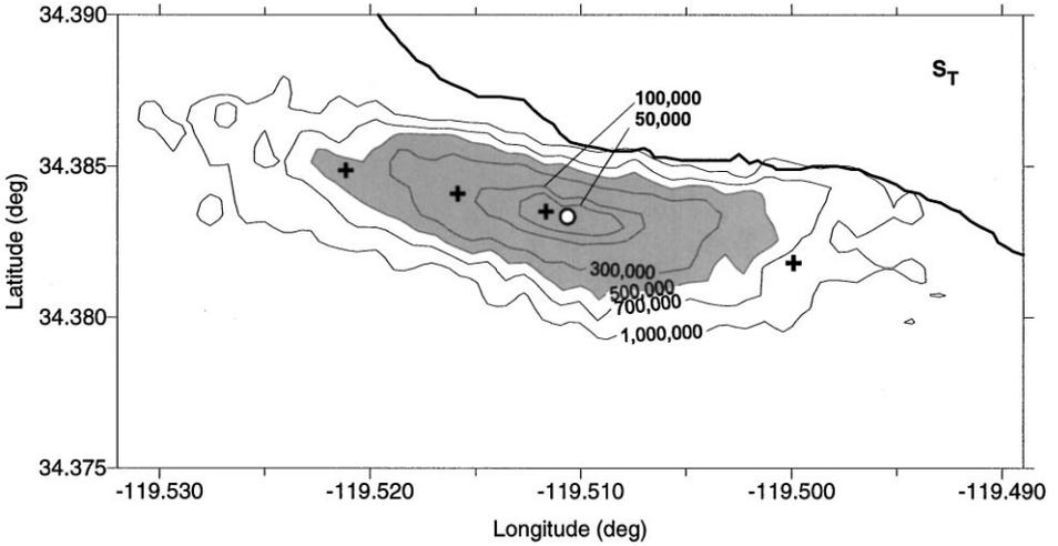
Fig. 10. (a) Time-averaged dilution in far-field  $S_T$  at 7 m depth.  $S_T$  is computed for summertime conditions, assuming near-field dilution  $S_m = 50$  and horizontal eddy diffusivity  $k_H = 5 \times 10^{-2} \text{ m}^2 \text{ s}^{-1}$ .  $S_T$  shown for visitation frequencies above 0.003. Time-averaged dilutions for wintertime conditions are 1–2 orders of magnitude larger (not shown).
