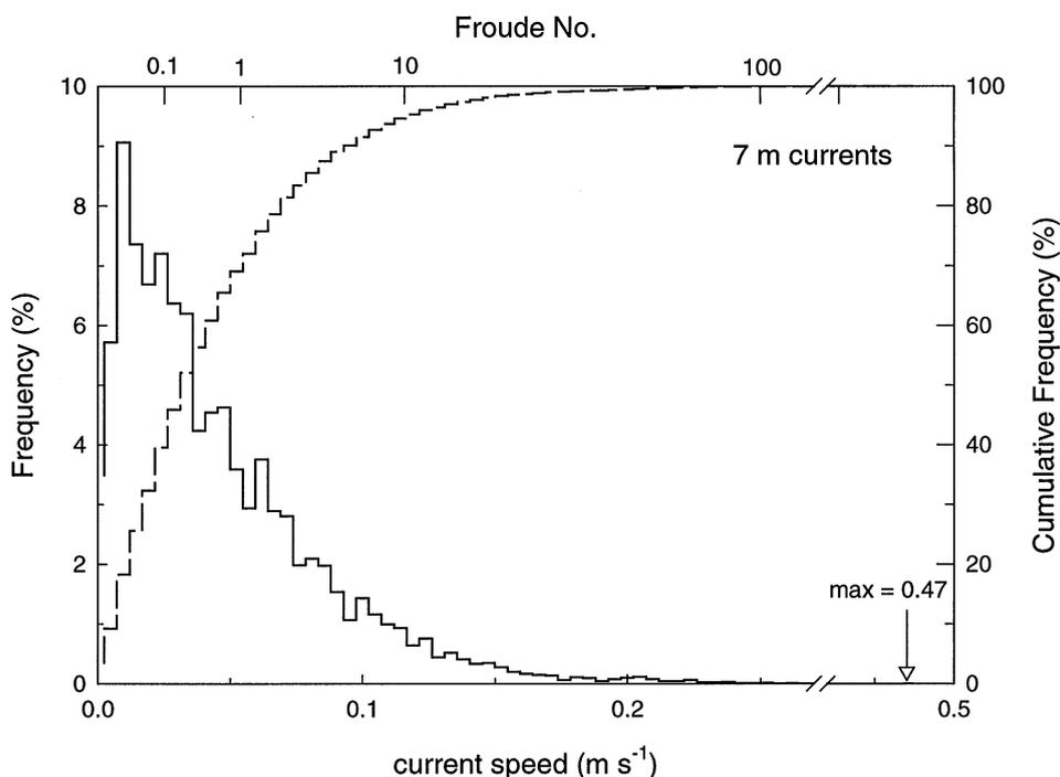
Fig. 6. Histogram (solid line, left hand scale) and cumulative distribution (dashed line, right hand scale) of current speed  $u$  at 7 m. Upper scale shows corresponding values of Froude number  $F = u^3 b^{-1}$  based on the mean specific buoyancy flux  $b = 1.56 \times 10^{-4} \text{ m}^3 \text{ s}^{-3}$ .
