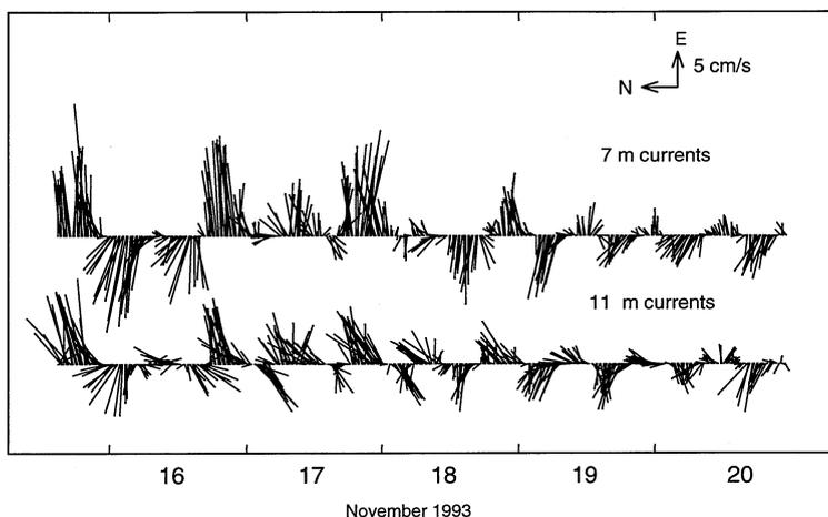
Fig. 4. Needle plots of current magnitude and direction at 7 m (upper time series) and 11 m (lower time series) for 16–20 November 1993. Each needle represents a 2 min vector average of a current velocity and needles are 20 min apart. Speed scale shown in upper right corner.
