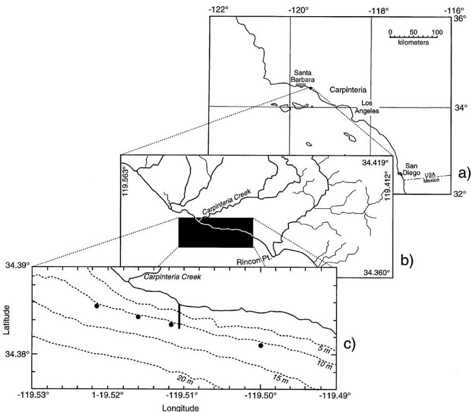
Fig. 1. (a) Area map of Southern California showing field site near Carpinteria, CA. (b) Map of coastline and watershed around the field site. (c) Field site showing produced water discharge pipe and diffuser (heavy line) and bathymetric contours (dotted lines). Dots indicate biological moorings at 100, 500 and 1000 m west of the diffuser and 1000 m east of the diffuser.
