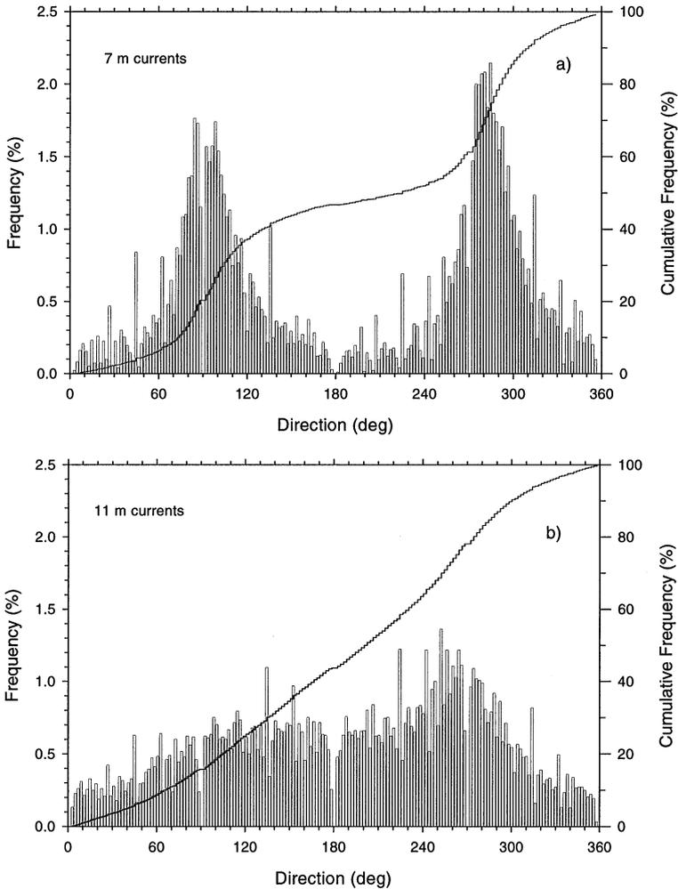
Fig. 5. (a) Histogram of current direction for 7 m data (left hand scale). Increasing curve shows cumulative frequency (right hand scale) Total of 17,337 points sorted. (b) As in (a) but for 11 m current direction. Total of 17,972 points sorted. Bin width is  $2^\circ$  in both histograms.
