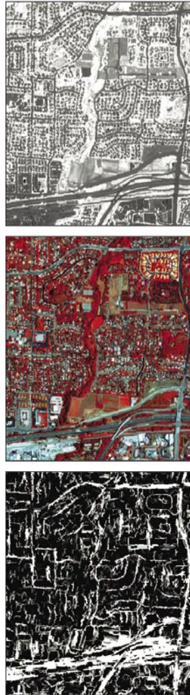
Figure 1: NDVI image subset (top), segmented image derived from IKONOS in channel 4,3,2 color composite (middle) and length/width ratio of the segmented image objects.
