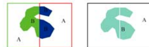
FIGURE 8.2: Steps in the dissolve operation. Left: Two maps show one feature, split across an edge. Attribute and graphic database have three records for type "B". Right: After dissolve, edge lines are removed and the three type "B" records are amalgamated.
