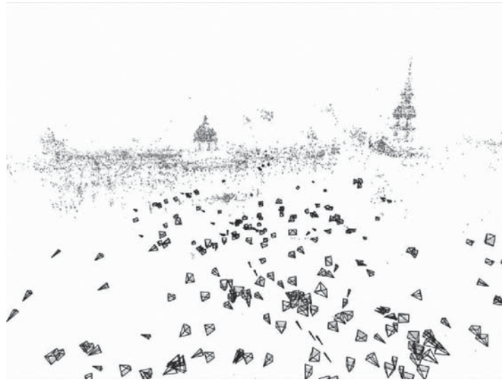
FIGURE 19.7 The Bundler open source image reconstruction software used to create a 3D point cloud from tourist photos of London's Trafalgar Square. (From Snavely, N. et al., Int. J. Comput. Vis. , 80, 189, 2008. With permission.)
