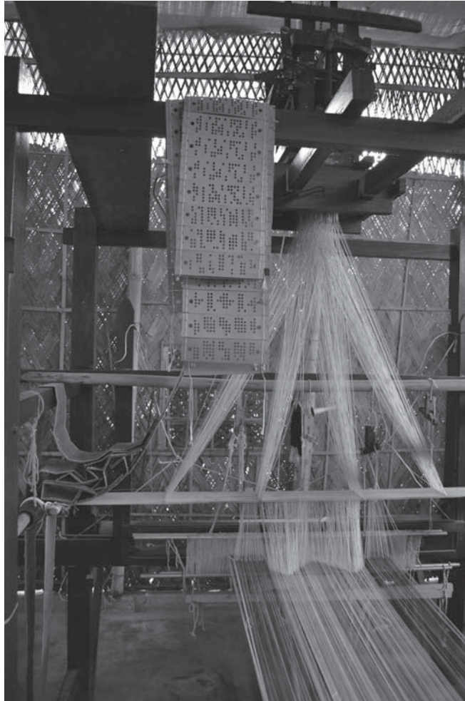
AQ3 FIGURE 19.2 Jacquard's weaving loom of 1805, found still in use in Assam, India. (Author.)
