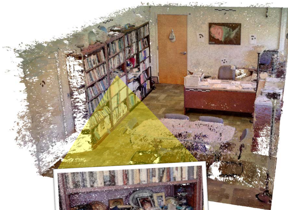
Raw 3D Point Cloud of EH Room 1720
