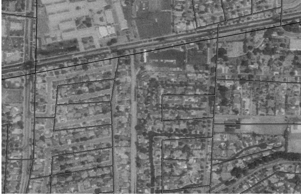
Figure 4. Misregistration of digital orthoimagery and roads in the US Geological Survey's National Map service.
