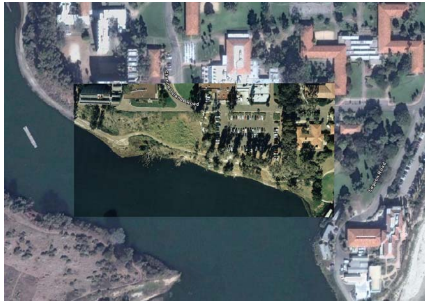
Figure 1: Mashup of a high-resolution image with Google Earth. Note the approximately 15m offset of the Google Earth base imagery, and the close agreement between the Google Earth roads layer and the high-resolution image.
