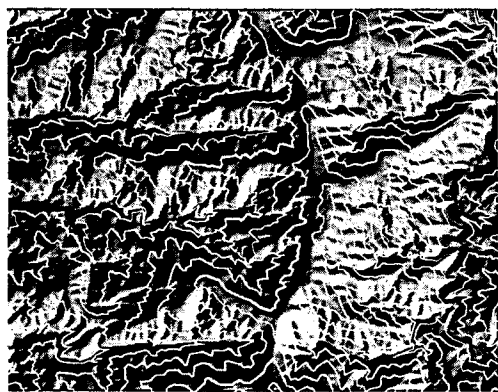
Figure 5a (top left): Showing the mean L H difference file after 10 realisations at p = 0.20 , with cells below and above the \pm 2 standard deviation threshold shown as white and black colour respectively.
