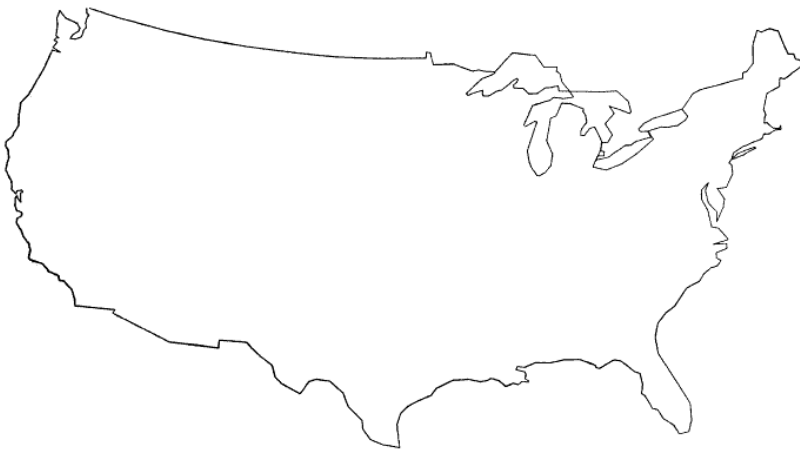
FIG. 7—Map of the United States drawn directly by machine from a deck of 343 punched cards. Plotting time, approximately 15 minutes. The map has been reduced, but not retouched. Bipolar oblique conic conformal projection (outline of original map from the American Geographical Society's Map of the Americas, 1:5,000,000). (Plotter courtesy the Benson-Lehner Corporation, Los Angeles.)
